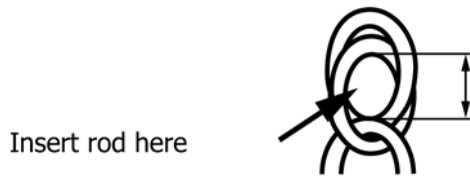
FIG. A1.26 Chain Criteria for Toddler Swings
