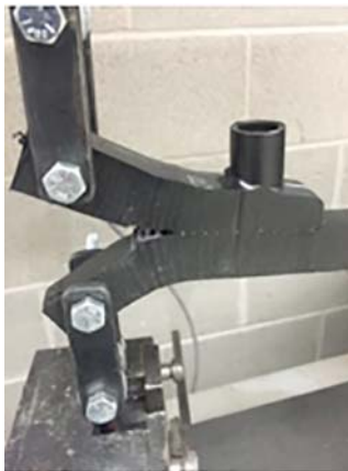
FIG. A2.4 Ductile Failure between Wires-Passing Result
