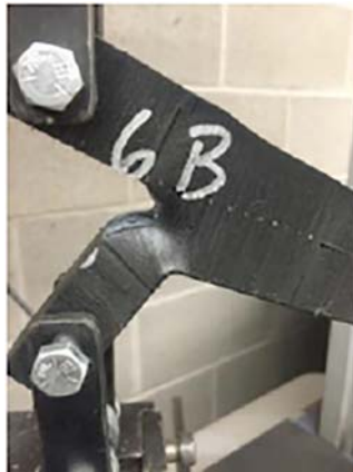
FIG. A2.3 Ductile Failure in Pipe-Passing Result
