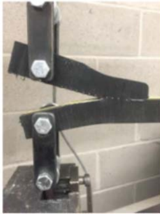
FIG. A2.5 Brittle Separation of Fusion Zone-Failing Result
