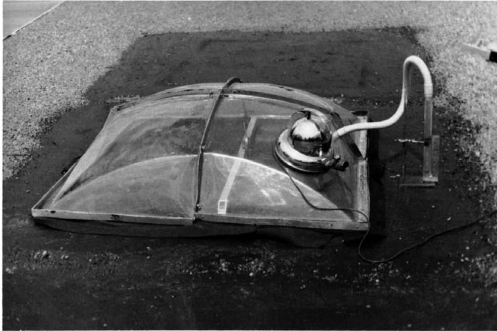
FIG. 1 View of Chamber over Roof Test Area During Test
