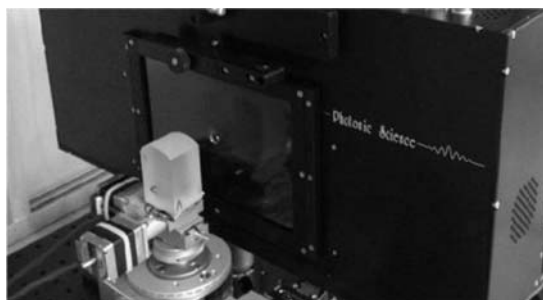
FIG. 1 Back-Reflection Laue Camera Measuring Sapphire Single Crystal Mounted on a Five-Axis Motorized Goniometer
