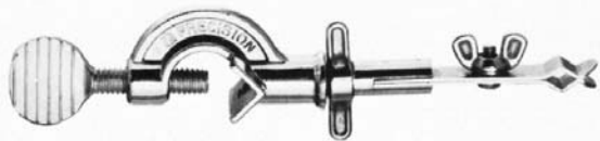
FIG. 4 Type IV—Thermometer Clamp
