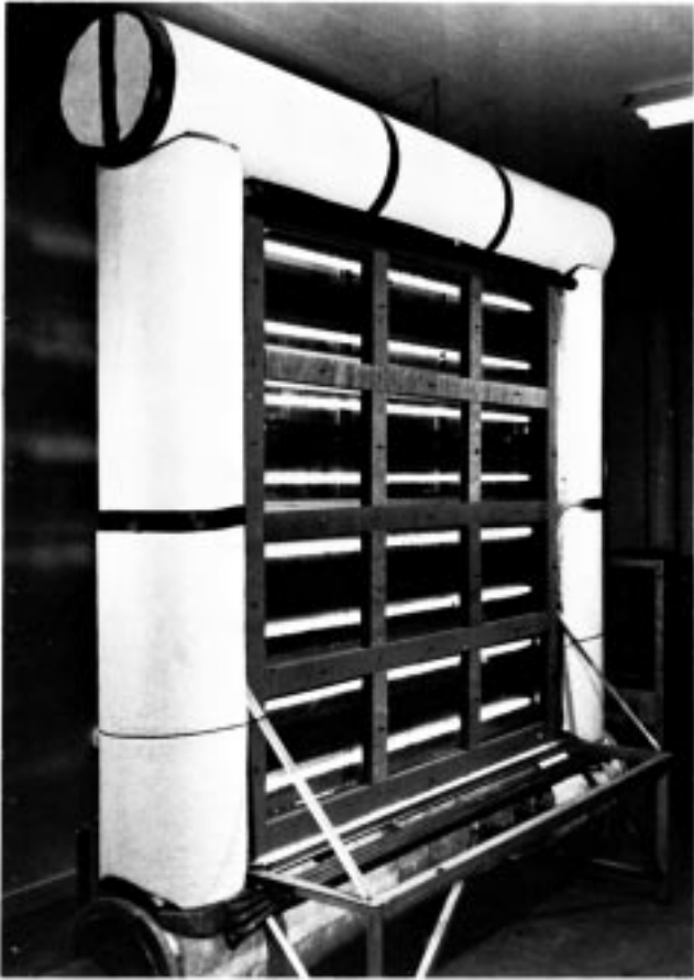
FIG. 1 Typical Accelerated Weather Cycle Test Apparatus
