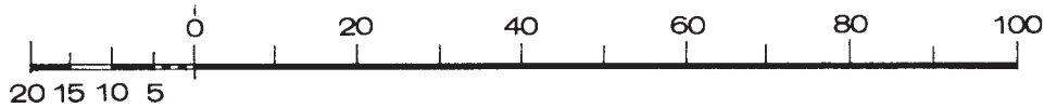
FIG. 1 Example of a Graphic (Drawn) Reference Scale for Drawings Likely to be Reproduced at a Different Scale Ratio
