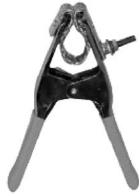
FIG. 7 Spring Loaded Contact Clamp
