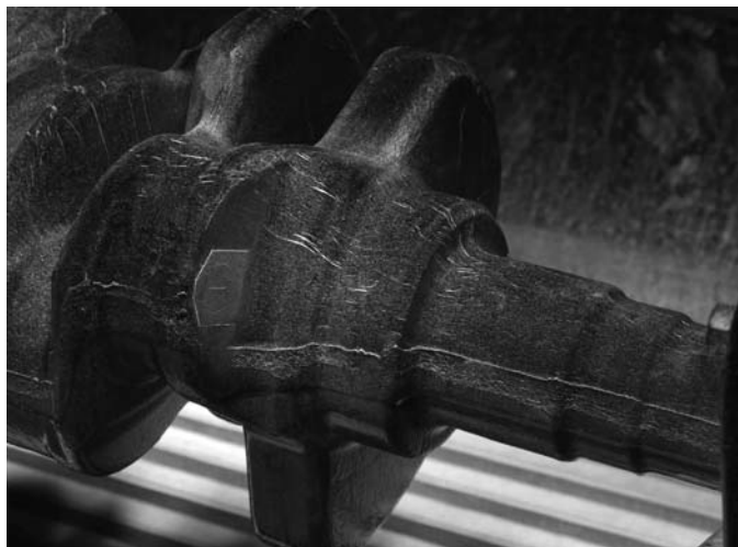
FIG. A1.4 Crankshaft with Various Longitudinal Indications
