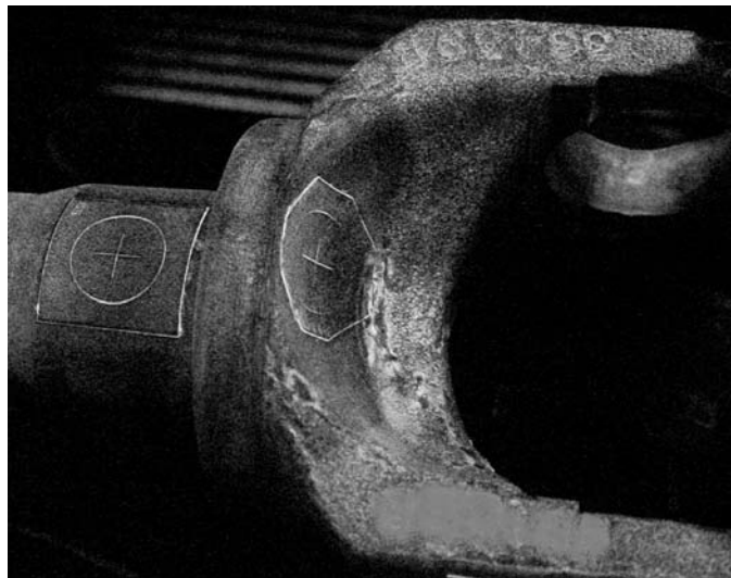
FIG. A1.6 Yoke Showing Balanced QQIs
