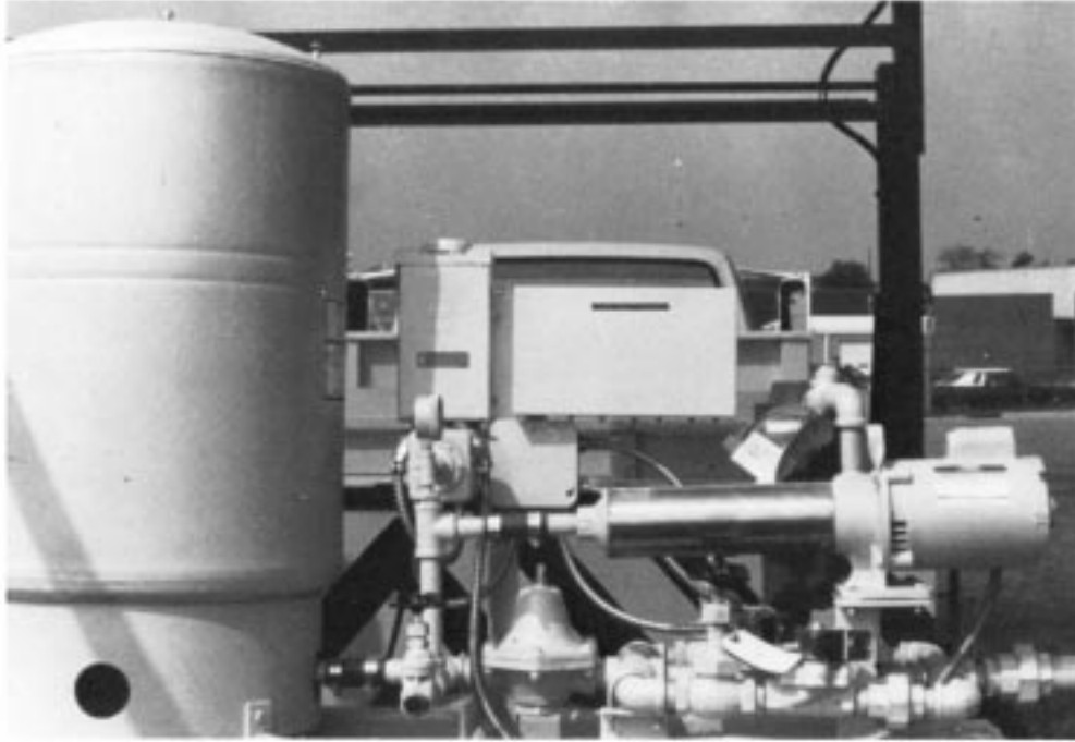
FIG. 2 Variable Speed Friction Tester Water System
