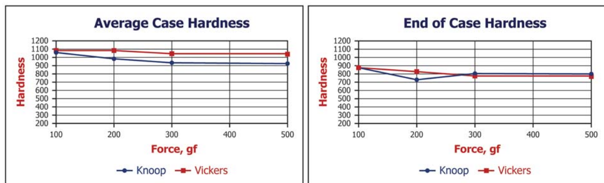
FIG. X5.13 Plots of the average case hardness (left) and the hardness at the end of the dark-etching case at ~0.14 mm (right) for the nitrided H13 mold. For HV values of 900 and greater, the conversion chart (Table 1 of E140) shows lower HK numbers; while the reverse is shown for HV values <900.
