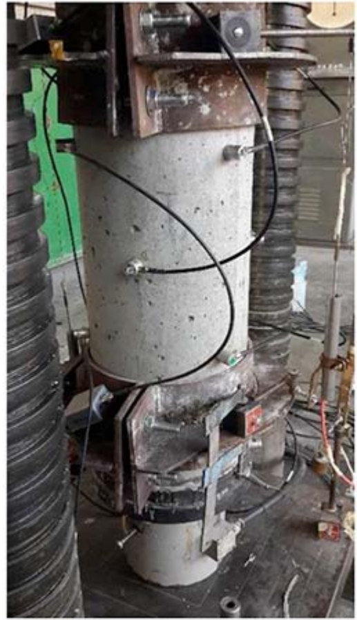
FIG. 2 Reinforced Column Specimen During Compression Testing
