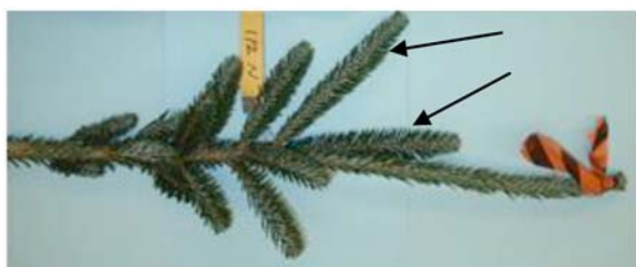
FIG. 3 A 2-year-old Branch Specimen with Arrows Showing a Pair of Current-Season Shoots to be used for Moisture Content and Fire Tests
