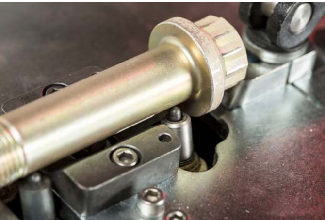
FIG. 5 Aerospace Fastener Test Nest
