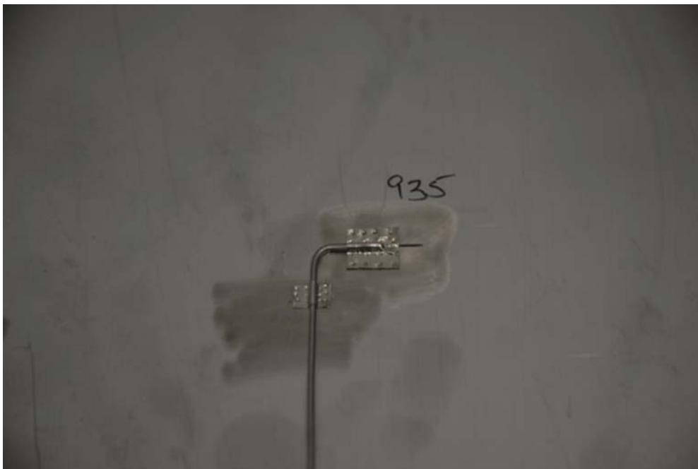
FIG. 3 Photo of Typical TC Installation
