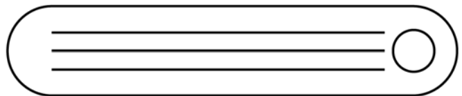
FIG. A3.1 The longitudinal lines represent the location of the slots cut into the center steel layer of either the General or Aerospace flexible laminated strips.
