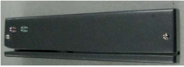
FIG. 5 Example of a Custom Skimmer (Door)
