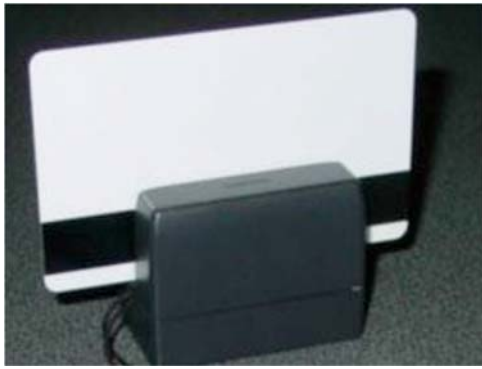
FIG. 1 Example of a Hand-Held Skimmer
