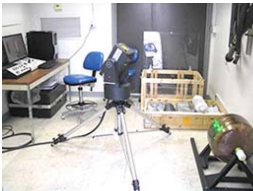
FIG. 13 Shear Camera Positioned Approximately 0.9 to 1.2 m (36 to 46 in.) from the Target COPV
