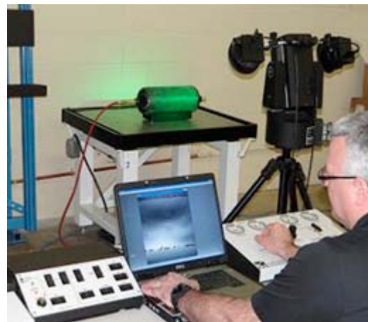
FIG. 12 Scan Plan for a COPV Involving Testing of the End Domes in Four Quadrants
