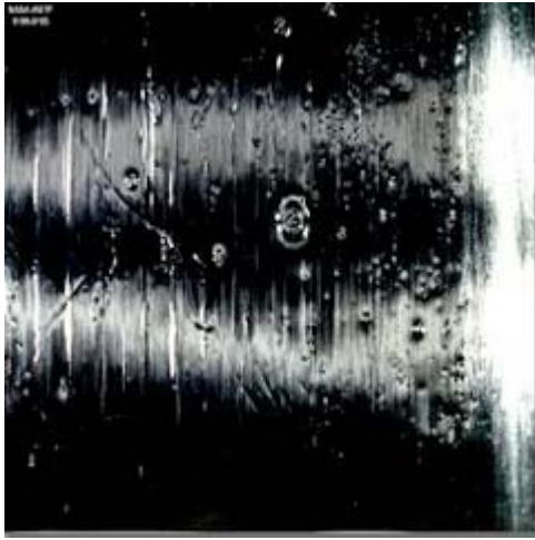
FIG. 28 Level I Resin Outgassing/Bubbling
