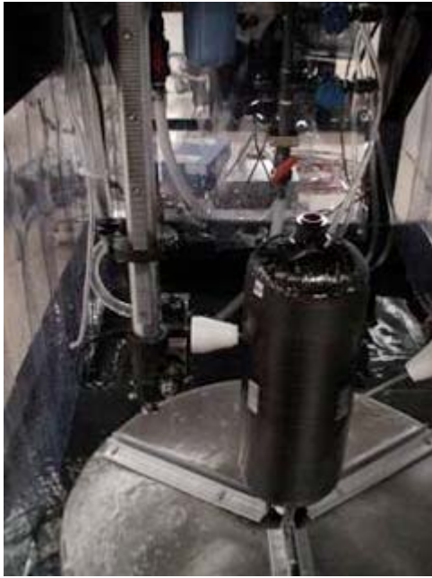
FIG. 26 Carbon-epoxy COPV in UT C-scan Pulse Echo Test Configuration using Water-jet Probes
