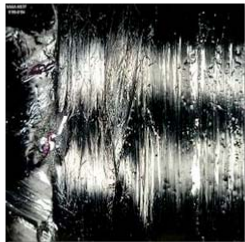
FIG. 27 Level I Manufacturing Artifact (Tow Termination)
