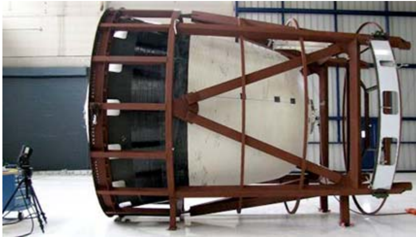
FIG. 11 A Large Carbon Fiber Reinforced Propellant Tank with a 4-m (13-ft.) Diameter Tested with a Maximum Pressure Loading of 0.7 kPa (0.1 psi)
