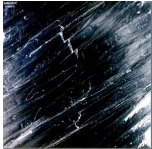
FIG. 32 Level II Broken Fiber Tows
