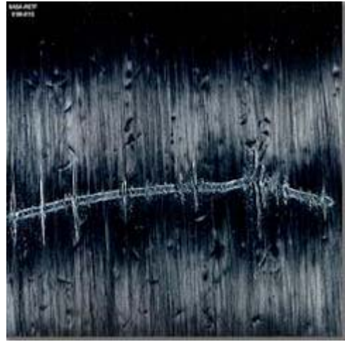
FIG. 31 Level II Scratch
