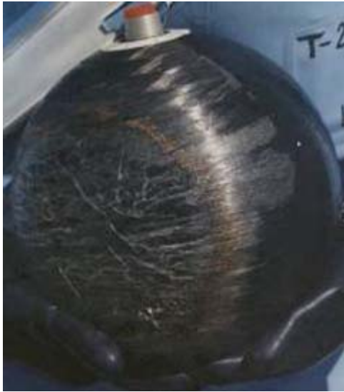
FIG. 33 Level II Discoloration (Propellant Exposure)
