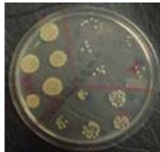
FIG. X3.2 Petri Plate Showing CFU of Staphylococcus aureus in the Drops from Undiluted Suspension and Two Serial 10-fold Dilutions
