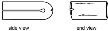
Flattened bend - outer surface and edge cracks
