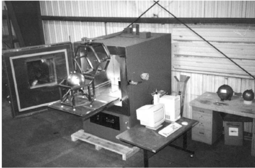
FIG. 3 Picture of Halon Bottle Test System Showing Oven, AE System, Halon Bottle on Oven Shelf.
