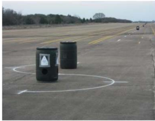
Left: The line-of-sight range test method uses an airstrip or paved road with robot test stations placed every 100 m (330 ft) along the centerline. Right: Robot test stations are prototyped with targets on the barrels for visual inspection tasks and circular paths for maneuvering tasks.
