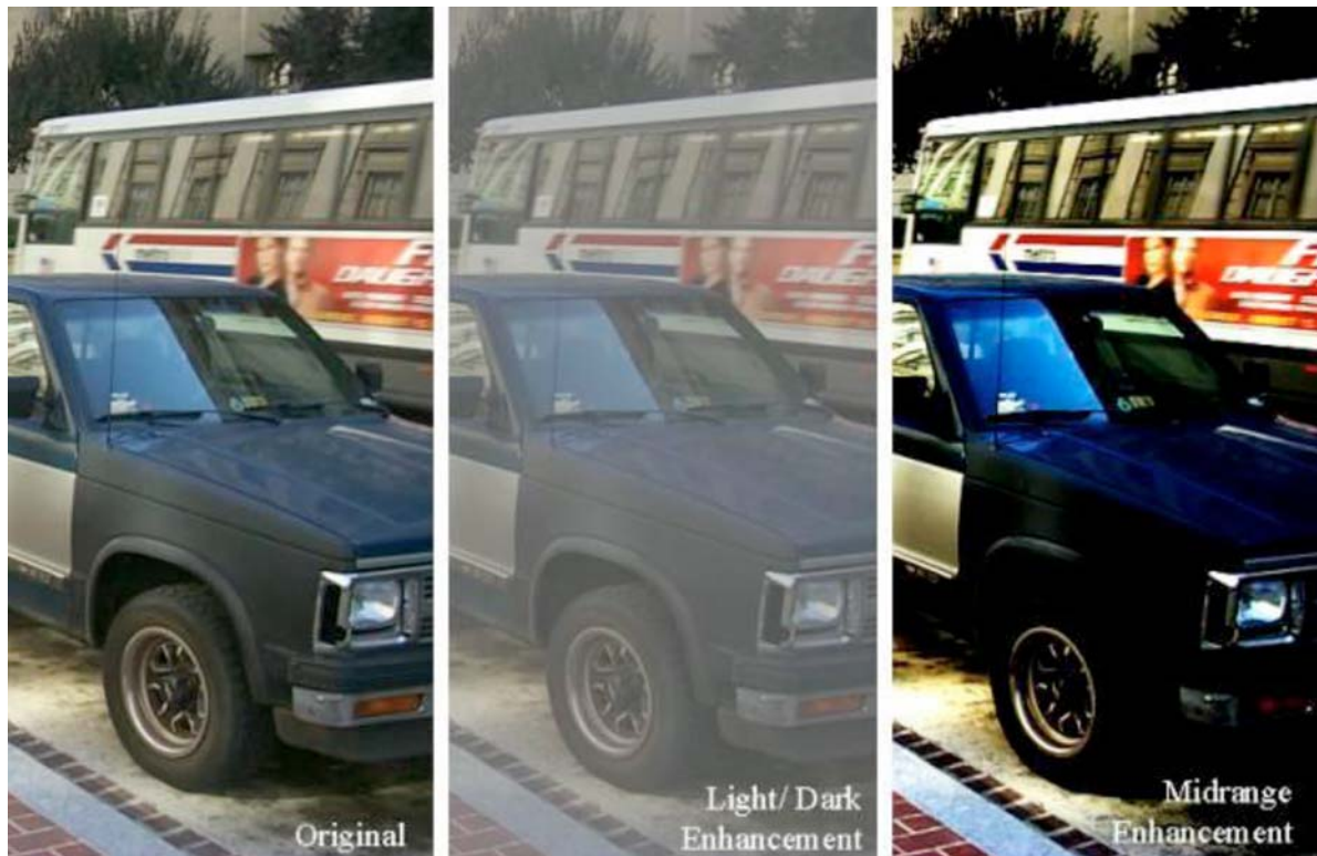
FIG. 2 This Example Shows Nonlinear Contrast Adjustments—Left: Original Image, Middle: Enhancement of Shadow and Highlight Areas at the Expense of Midrange Tones, and Right: Enhancement of Midrange Tones at the Expense of Shadow and Highlight Areas
