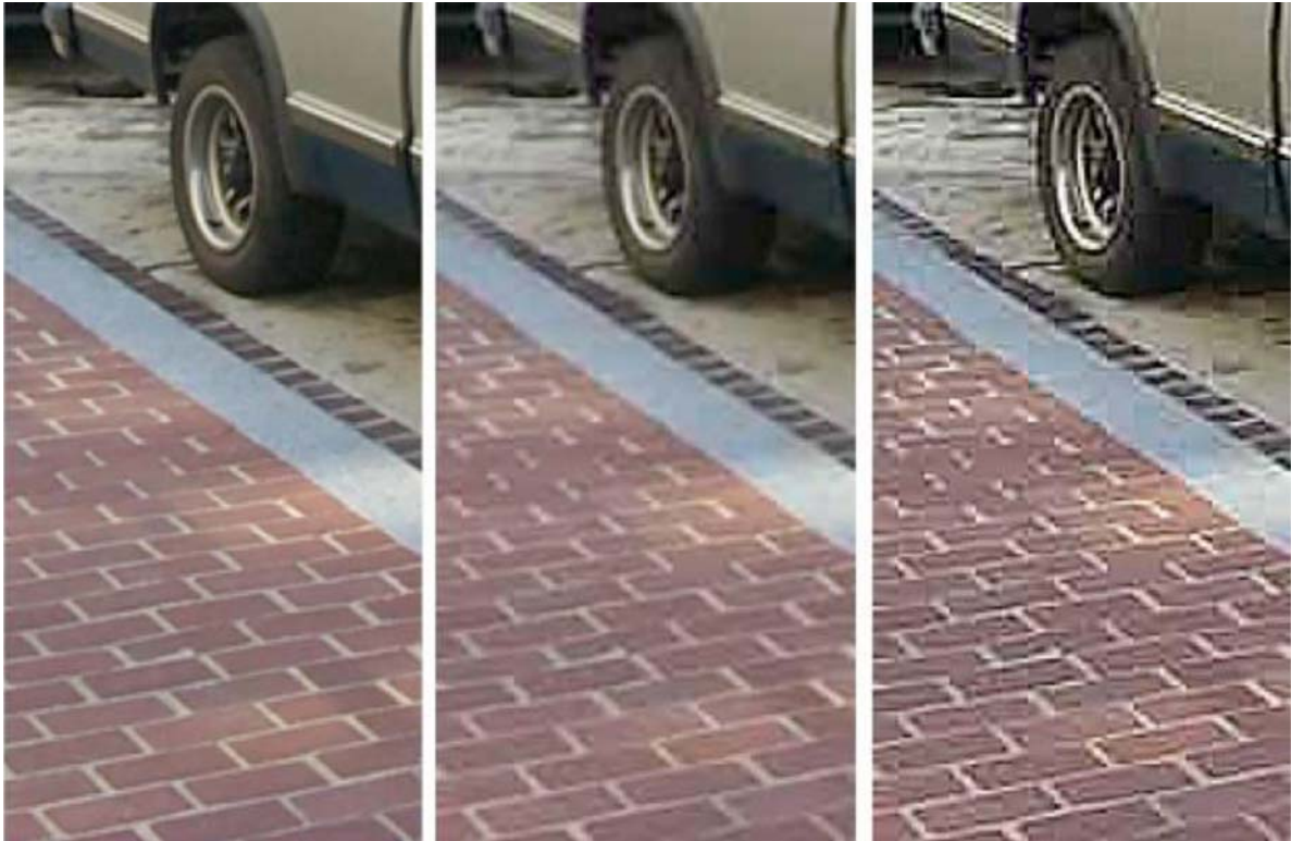
FIG. 3 Left: Original Image, Middle: the Result of JPEG Compression (Compression Ratio = 15:1), and Right: the Result of Edge Enhancement after Compression
