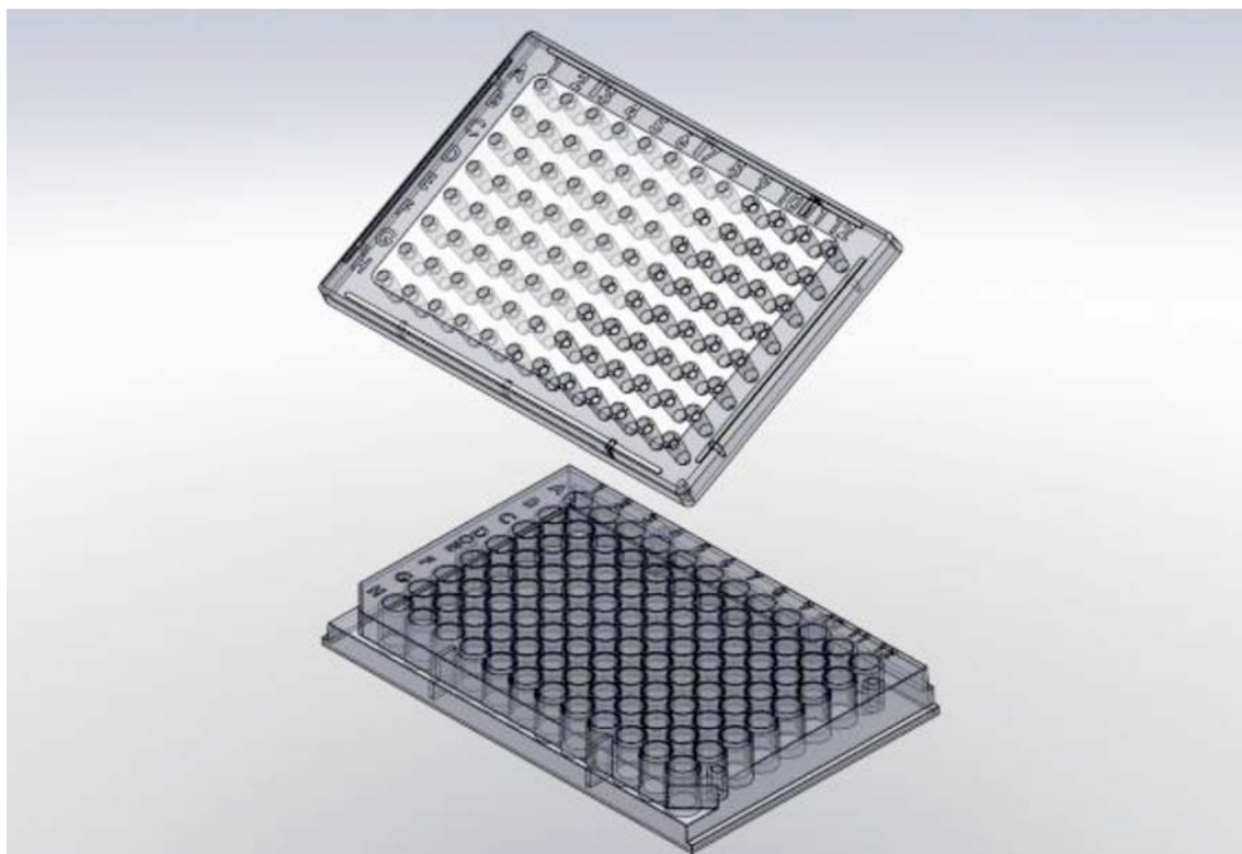
96-well tissue culture plate (bottom) and corresponding 96-peg lid (top).
