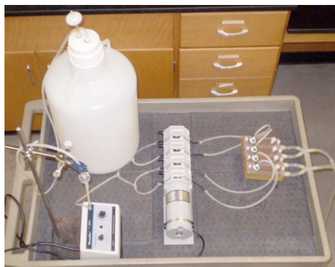
FIG. 2 Drip Flow Reactor Laboratory Set-Up in Continuous Flow Operation
