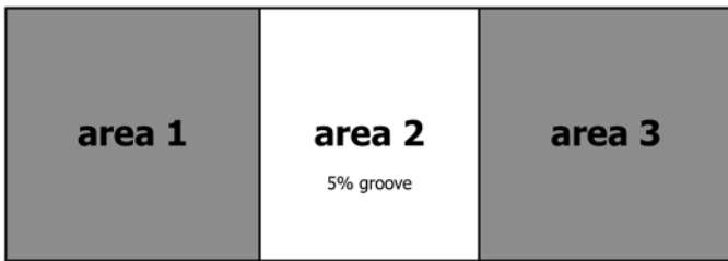
FIG. 6 Areas on the Step-Wedge Marked as Area 1, Area 2, and Area 3, which will be Used for Extracting Signal and Noise
