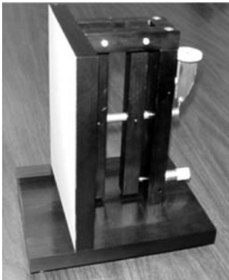
FIG. 3 A shearography camera calibration device consists of a means to apply a known deformation to an aluminum flat plate. The flat surface deformation is imaged. This device allows verification of the shearography camera operation, laser stability, and the minimum coherence length.
