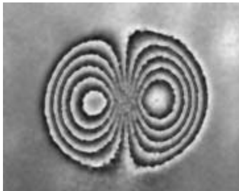
FIG. 4 A Phase Map Shearogram of a Reference Standard Consisting of a Plate with a Flat-Bottom Hole Using a Horizontal Shear Vector
