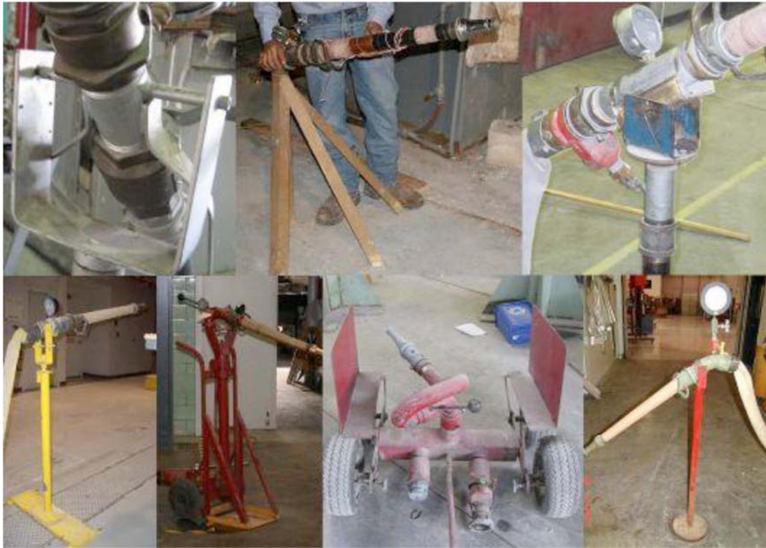
FIG. 2 Typical Hose Mounting Methods
