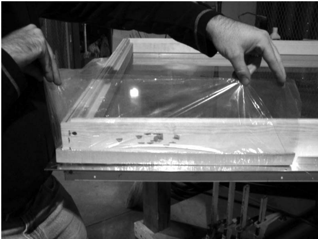
FIG. A1.8 Type B Material Applied with Polyethylene Liner
