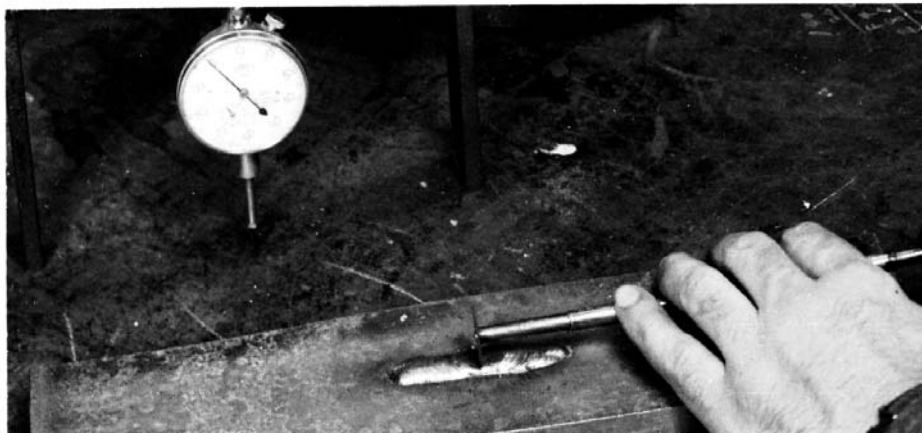
FIG. 8 Notching of Crack-Starter Weld Deposit
