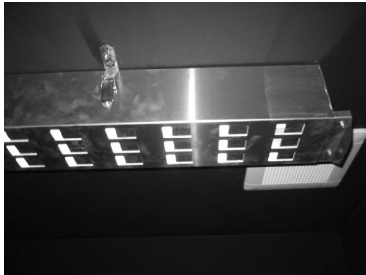
FIG. X3.1 Example of a Baffling System
