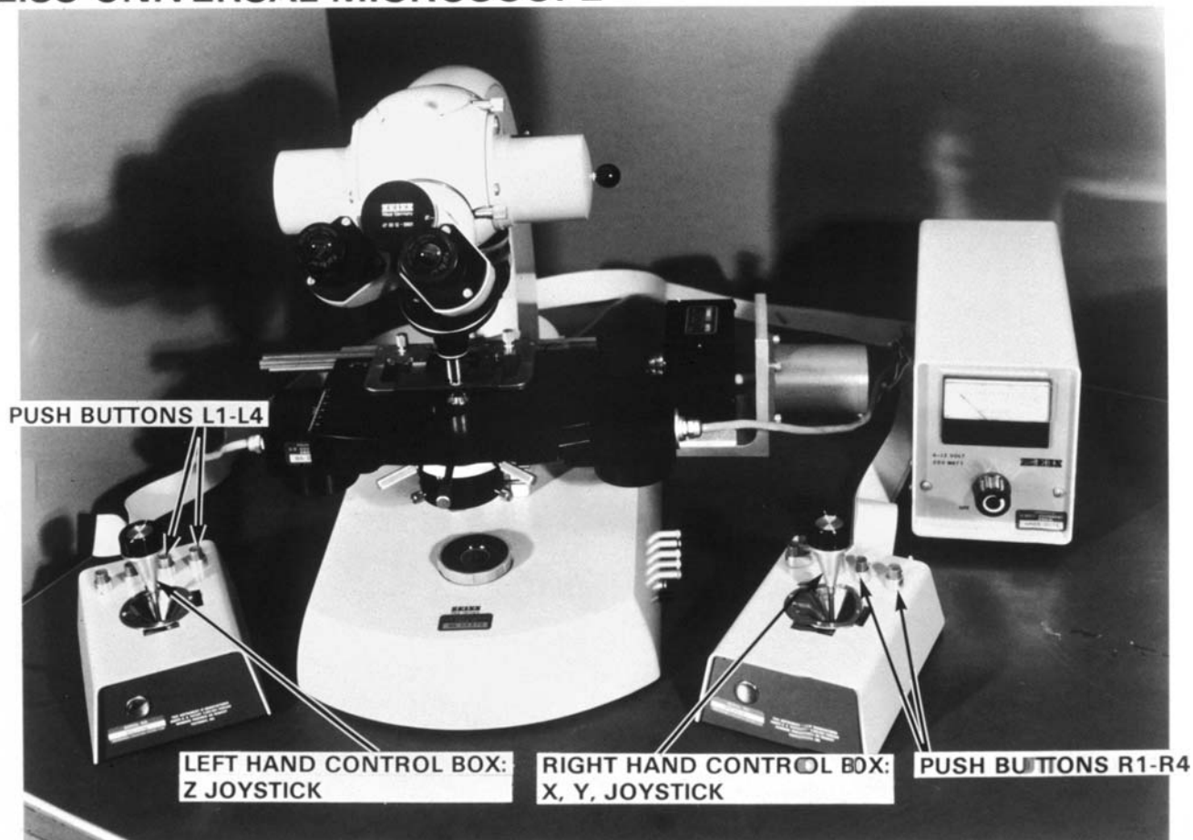
FIG. 5 Close Up of the ESP Microscope Showing Push Buttons and Stage Controls
