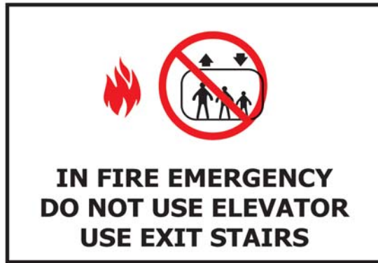
FIG. 9 Do Not Use Elevator Sign
