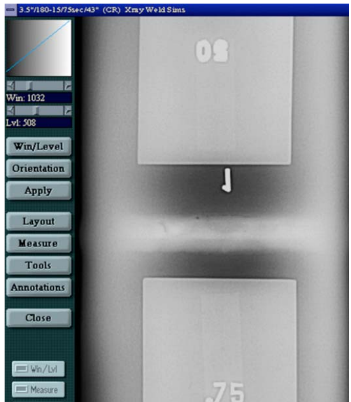
FIG. 26 Pipe Weld Features with Moderate Win-Levels
