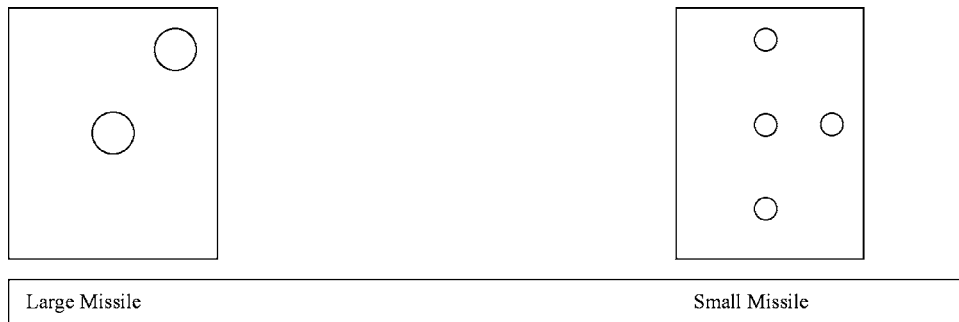
FIG. A1.2 Single Specimen Impact Locations
