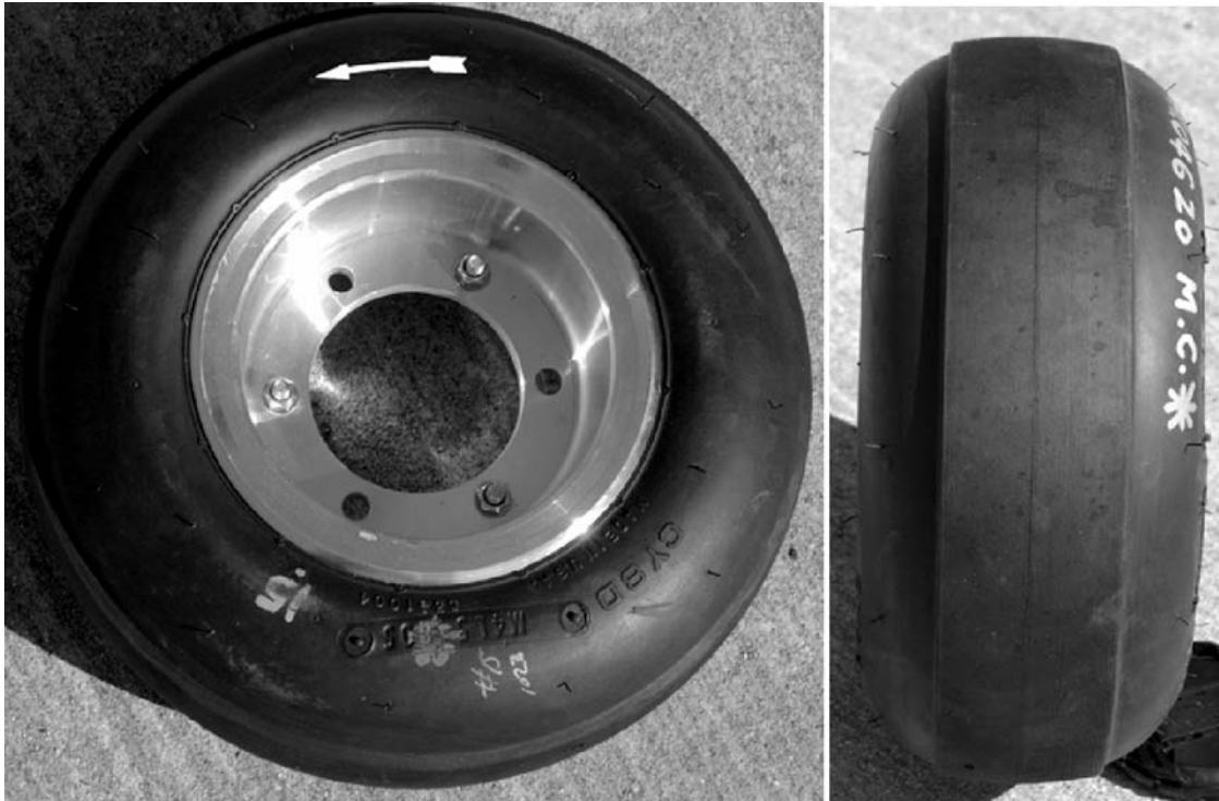
FIG. 1 Molded on Tire: 10 × 4–5 Tread ASTM Batch No.
