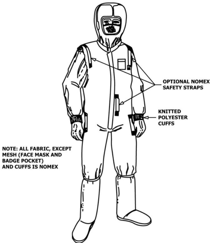
FIG. 6 Special Features of the Nomex Garment Ensemble
