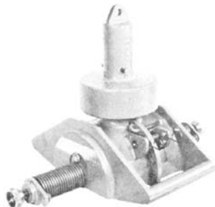
FIG. A1.7 Shipek (Scoop) Grab (Photograph courtesy of Hydro Products.)
