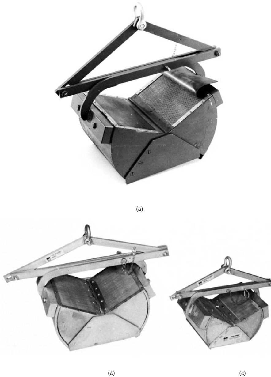
FIG. A1.1 Ponar Grabs. (a) Screen-Top Sediment Grab, Standard Design (Photograph courtesy of Kahl Scientific Instrument Corp.); (b) Screen-Top Wildco Ponar Grab, Standard Design; (c) Wildco Petite Ponar Grab (Photograph courtesy of Wildlife Supply Co.)
