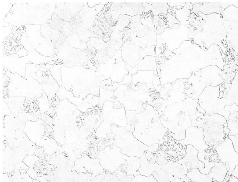
FIG. 1 Example of Replica Microstructure at 100x LM. Material: See Specification A335/A335M, Grade P22. Etchant: 2 % Nital
