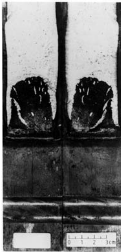
FIG. A1.11 Fracture Surface of a CCA Specimen with an Unacceptably Tunneled Crack Front
