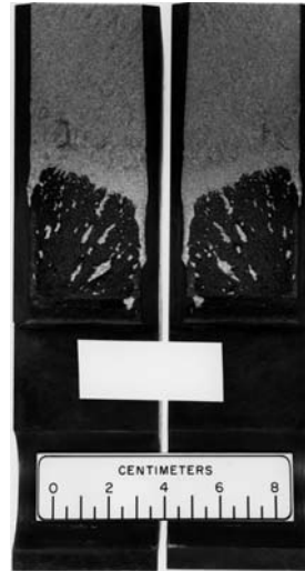
FIG. A1.10 Fracture Surface of a CCA Specimen with a Tunneled but Acceptable Crack Front
