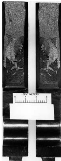
FIG. A1.4 Fracture Surface of a CCA Specimen Showing a Large Remaining Ligament Aligned with the Direction of Crack Propagation
