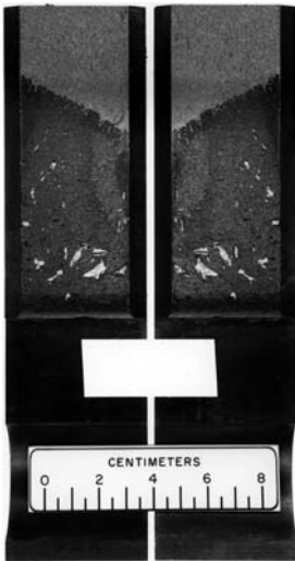
FIG. A1.8 Fracture Surface of a CCA Specimen with a Slanted and Straight Crack Front
