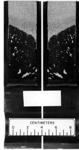
FIG. A1.9 Fracture Surface of a CCA Specimen with a Slanted and Nearly Straight Crack Front
