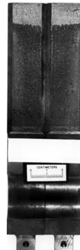
FIG. A1.2 Another Example of an Ideal Fracture Surface of a CCA Specimen
