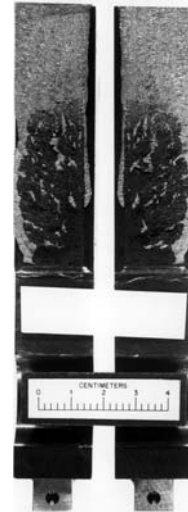
FIG. A1.13 Fracture Surface of a CCA Specimen for Which the Crack has Grown Out of the Midplane of the Specimen but has Remained Mostly Within the Net Specimen Thickness, B_N
