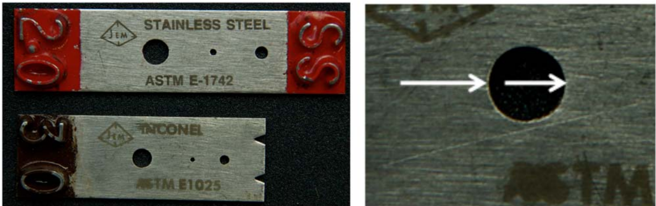
FIG. A1.1 ASTM IQIs for Measurement of Spot Size by Edge Evaluation
