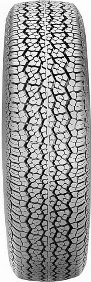
FIG. 1 Front View of the P195/75R14 Radial Standard Reference Test Tire
