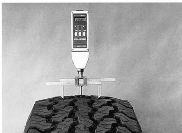
FIG. 5 Measuring the Tread Radius Using the Three Point Drop Method
