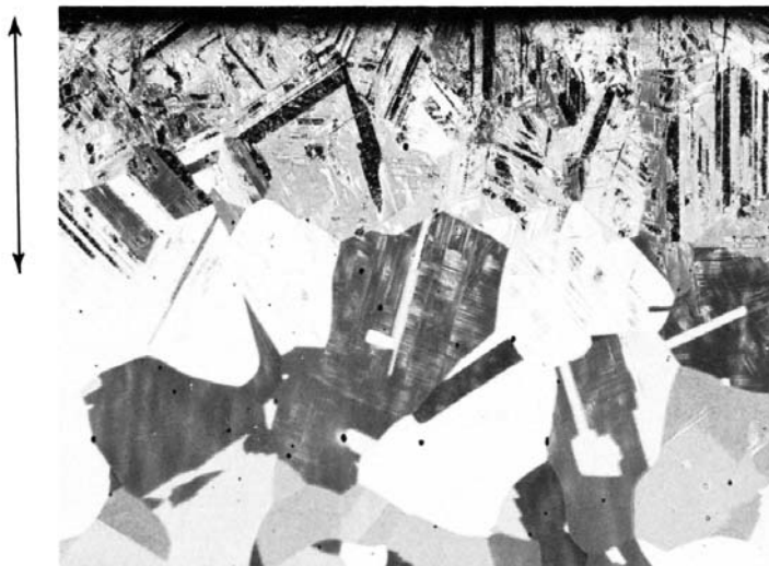
FIG. 10 Example of Epsilon Martensite Formation in the Decarburized Surface Zone of a Solution-Annealed Austenitic Manganese Steel Where the Carbon Content is Less than 0.5 % (100x, Etched With 2 % Nital for 5 s, then 20 % Aqueous Sodium Metabisulphite for 20 s)
