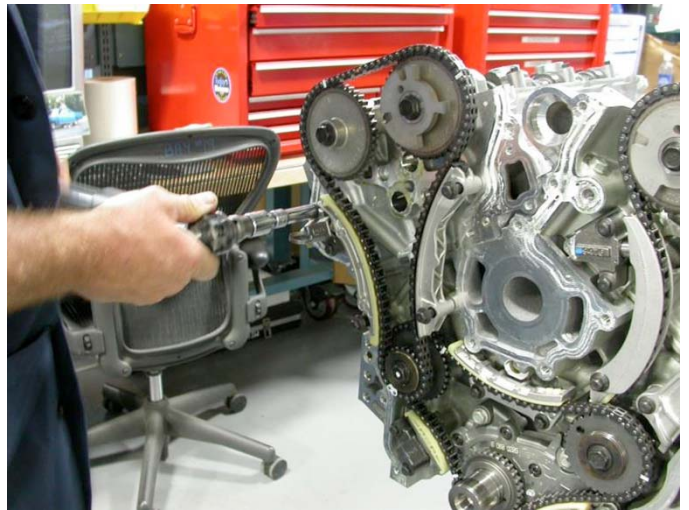
FIG. A17.12 View Showing Chain Guide and Tensioner Installation
