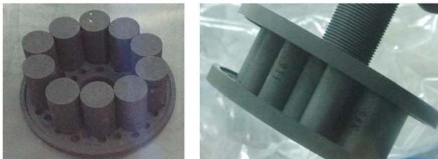
FIG. 2 Sample Holder: Graphite Plates and Sample Rod
