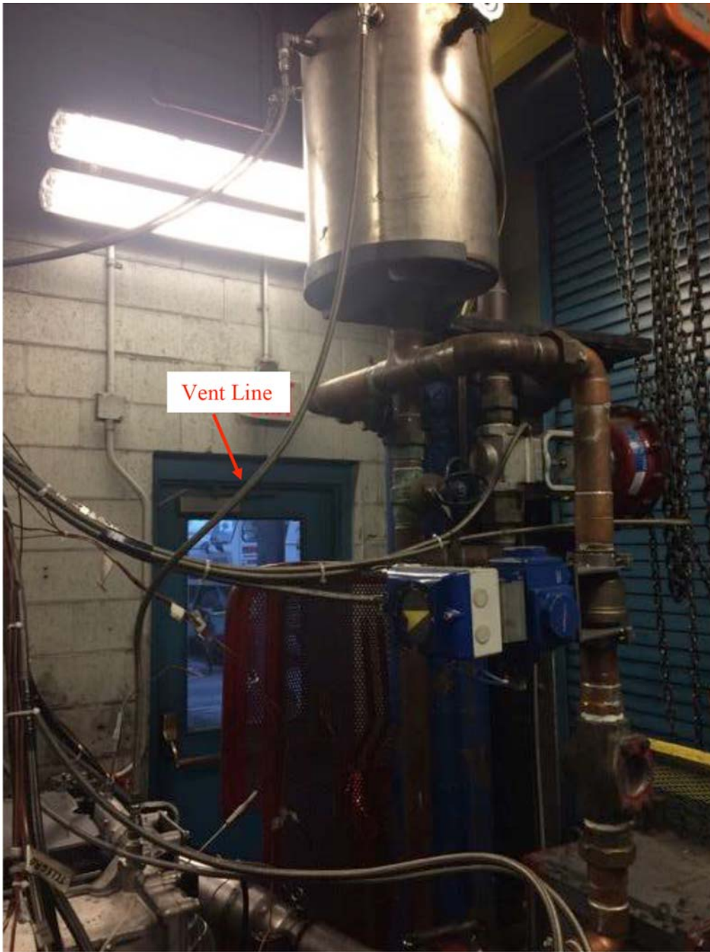
FIG. A4.3 EGR Cooler Vent Line and Coolant Tank
