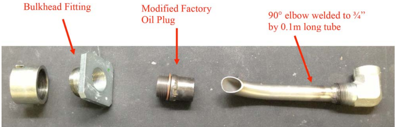
FIG. A4.6 Modifications to Oil Pan Bulkhead Fitting for Auxiliary Oil-System Suction Line
