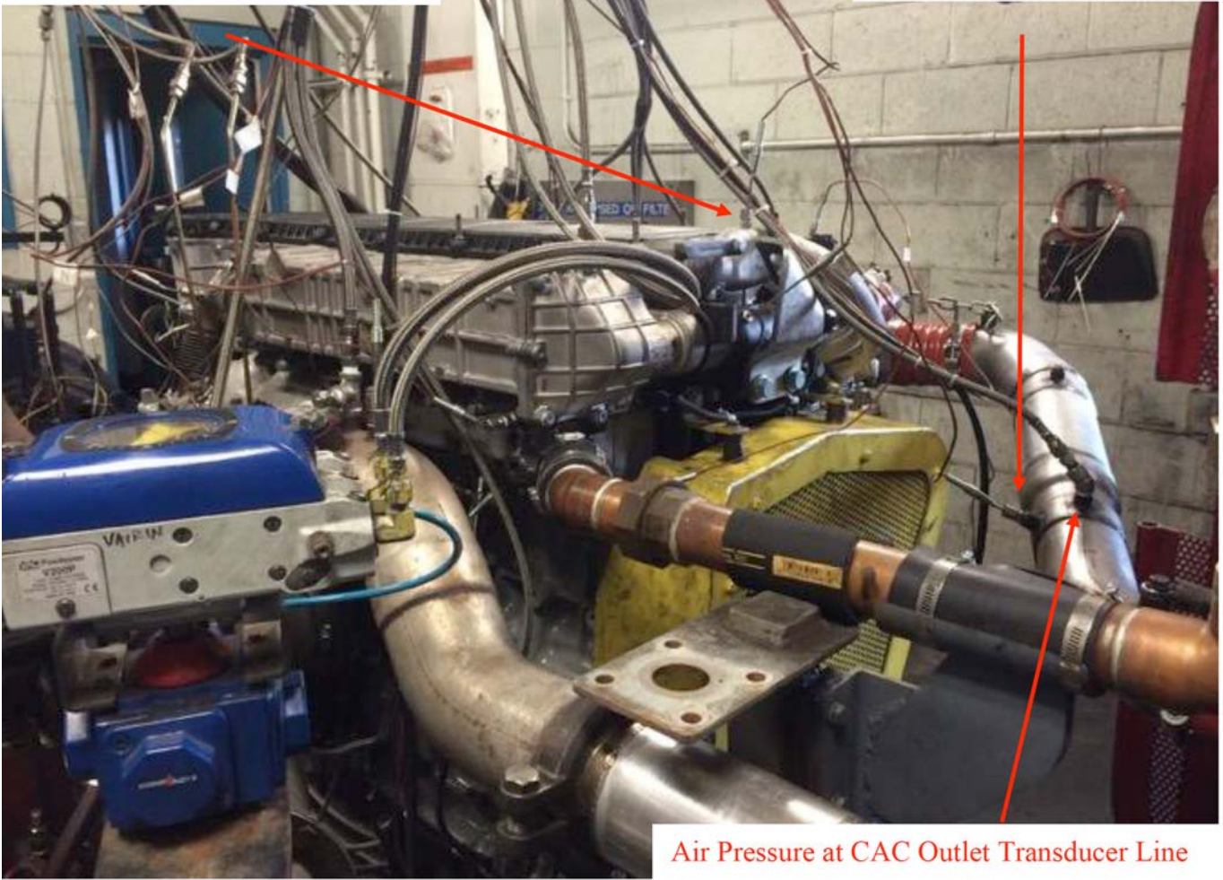
FIG. A4.22 Location of Sensors for Air Temperature and Pressure at CAC Outlet and Coolant Inlet Temperature to EGR Outlet Sensors
