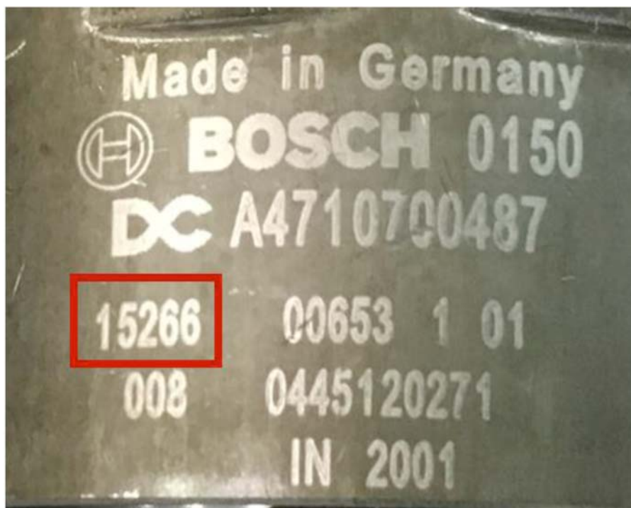
FIG. X1.1 Location of Date Codes for Injector Nozzles
