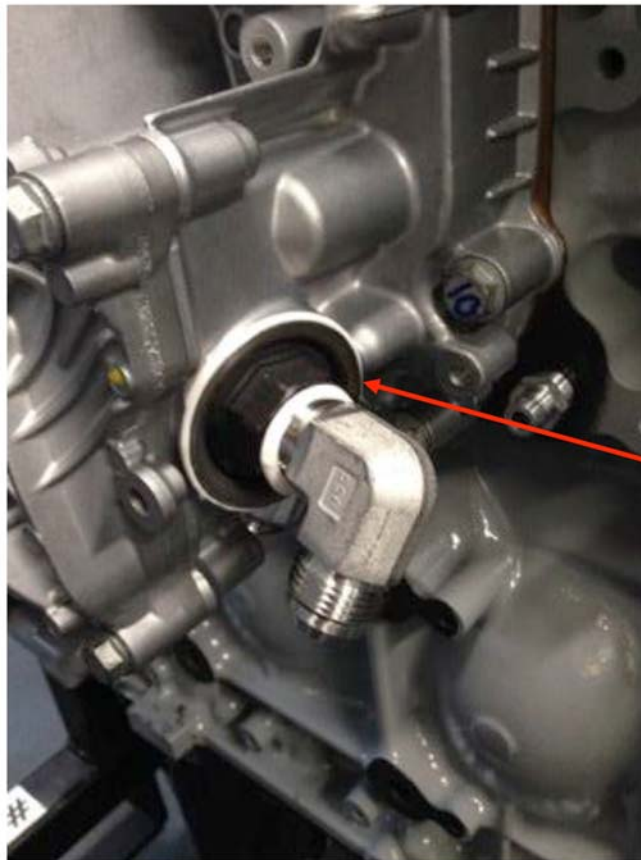
FIG. A4.13 Oil Module to Remote Oil Heat Exchanger Return Modification
