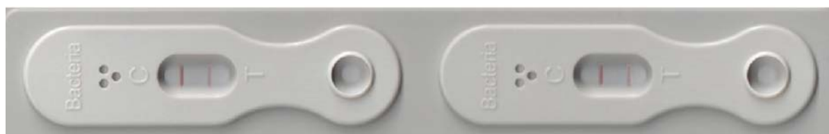
FIG. 3 Bacteria LFD Detecting ≤150 µg Antigen/L Fuel Phase or ≤33 µg Antigen/mL Aqueous Phase: Both Test and Control Lines Visible
