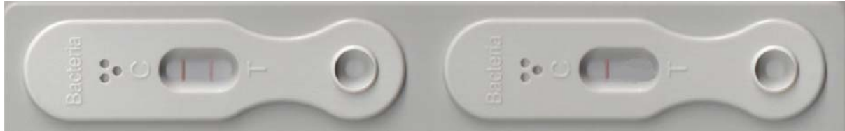
FIG. 4 Bacteria LFD Detecting >150 \mu\text{g} to \leq 750 \mu\text{g} Antigen/L Fuel Phase or >33 \mu\text{g} Antigen/mL Aqueous Phase and \leq 166 \mu\text{g} Antigen/mL Aqueous Phase: Test Lines are Visible Only on the High-Range (Left) LFD
