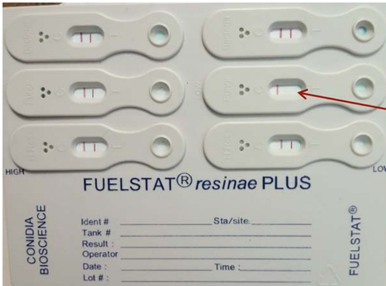
FIG. A1.2 LFD Tray Detecting >150 \mu\text{g} to \leq 750 \mu\text{g} Antigen/L Fuel Phase or >33 \mu\text{g} Antigen/mL Aqueous Phase and \leq 166 \mu\text{g} Antigen/mL Aqueous Phase in the Fungi LFD
