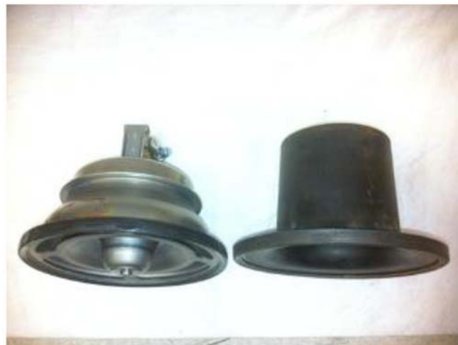
FIG. A6.1 Sleeve Replacing Thermostat
