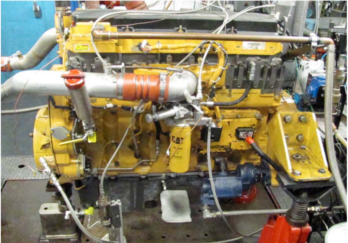
FIG. A5.20 Left-Hand Side of Installed Engine
