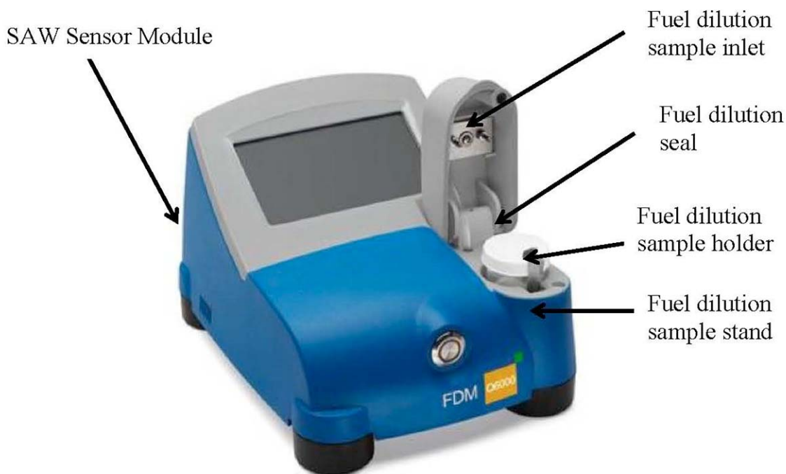
FIG. 2 Example SAW Fuel Dilution Apparatus—Configuration B
